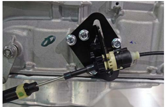
Figure 7: Install Cable to Bracket
