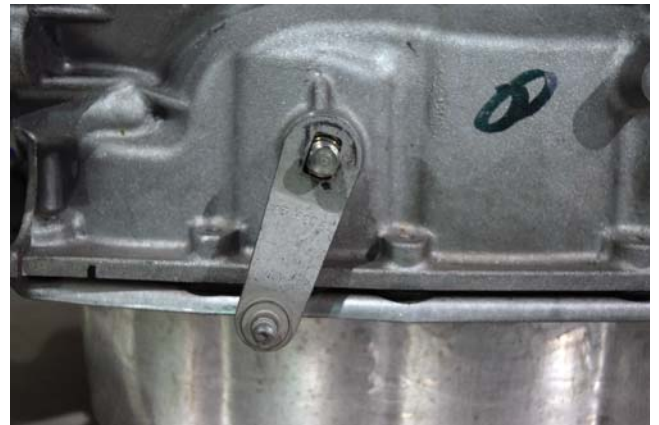
Figure 1: Install Shift Arm
