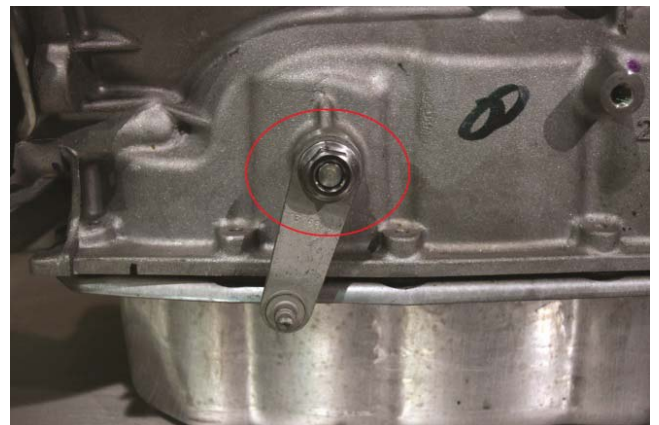
Figure 2: Install Shift Arm Nut
