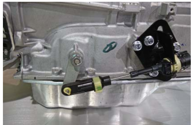
Figure 8: Install Cable End onto Shift Arm
