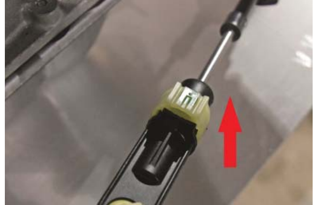
Figure 6: Release Cable End Adjustment
